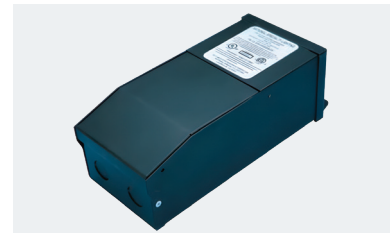
TR-24-960 12.5" x 7.0" x 4.75" 2 circuits at 480 watts each for 24V AC
