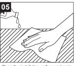
Clean the installation surface and make sure the surface to be installed is smooth and free of any dust or oil stains.
