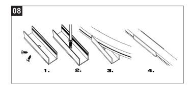
**NOTE:** For porous surfaces that will not allow a firm grip with the self adhesive backing, we recommend that you use our U channel (SL-OD-MC) or extrusion (SL-OD-EX-39). Scan QR Code below for more information on other extrusion options.
