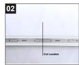
Measure the length of the surface where the LED strip is to be installed and cut on the closet cut location with sharp scissors.
