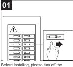
Before installing, please turn off the power supply to the circuit in use.
